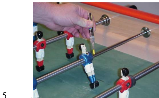
5. Apply 1 drop of lube to the inner rod We recommend Super Lube.
